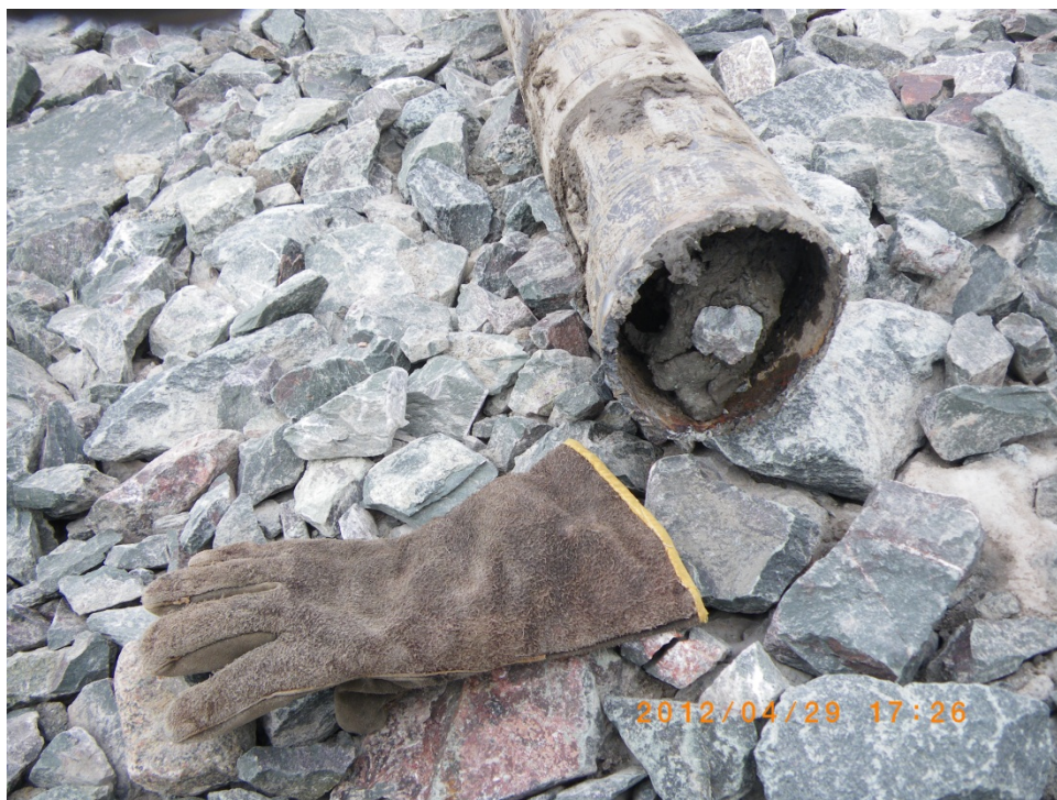
Photo 2: The crippled and cut steel casing. Overburden material was observed on the down-hole hammer rods and inside the steel casing.
